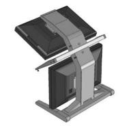
6. Remove the beamsplitter from the shipping case. With the StereoMirror™ logo oriented to the lower right, insert the pins located on either side of the mirror frame into the corresponding slots on the mirror support arms. The pins should rest in the fully forward position of the mounting arm slots.
